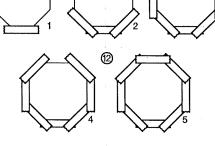
12. Tape over moisture barrier cut lines and exposed nails with flashing tape. \* for brickmould, tape along with a 3/4" overlap on brickmould.
