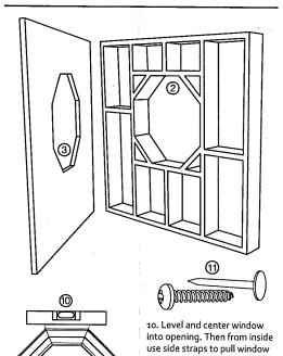
in tight and tack through straps to hold in place. 11. Secure into opening with screws or nails through side
